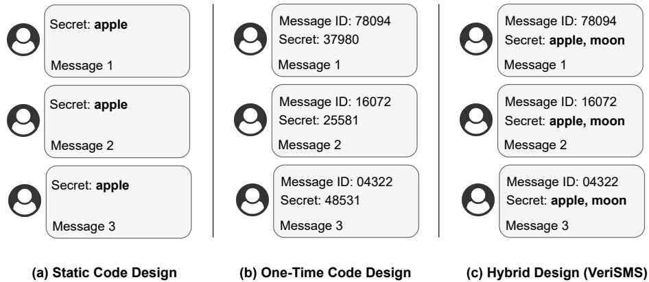
Figure 2: Example Messages —VeriSMS adopts a hybrid design to balance security and usability.
