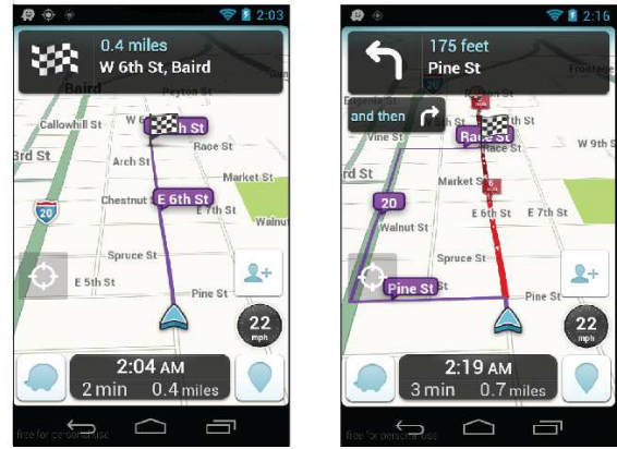
Fig. 1. Before the attack (left), Waze shows the fastest route for the user. After the attack (right), the user gets automatically re-routed by the fake traffic jam.
